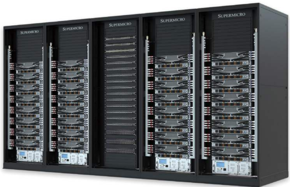
Liquid-Cooled AI SuperCluster With 256 NVIDIA HGX B200 GPUs, 32 4U Liquid-cooled Systems
